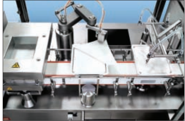
Figure 2: Fully automatic tub opening (ATO). Smooth and low particle opening process.
