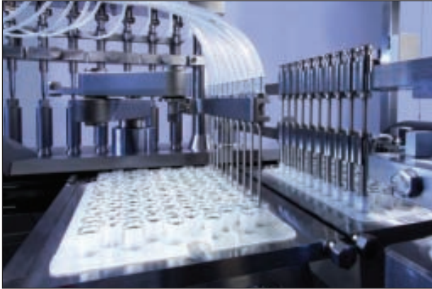
Figure 1: Filling and stoppering station FXS 5100. Provides continuous filling and stoppering without any interruption during the change of the nest.
