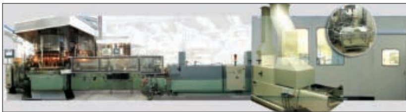
Figure 1: The S.P.A.M.I. barrel-forming line leading to the controlled environment area.
