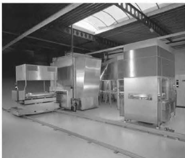
Figure 11 Lyophilizer transfer cart with loader and unloader (13).
