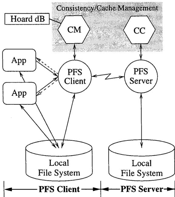
Figure 2: Block diagram of PFS.
