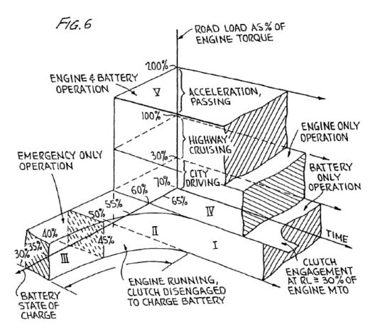
Figure 6 illustrates differing modes of vehicle powertrain operation, plotted on a three dimensional chart, illustrating that the mode of vehicle operation is a function of the state of charge of the battery bank, the instantaneous road load, and time. *Id.* at 21:53–57.
