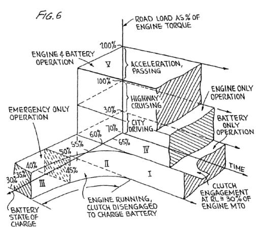
Figure 6 is a three-axis schematic with time on one axis, road load on a second axis, and battery state of charge on the third axis, illustrating that the mode of vehicle operation is a function of the state of charge of the battery bank, the instantaneous road load, and time. *Id.* 21:53–57.
