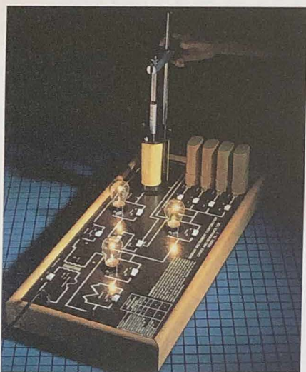
This versatile circuit enables the experimenter to examine the properties of circuit elements such as capacitors and resistors and their effects on circuit behavior. (Courtesy of Central Scientific Company)
