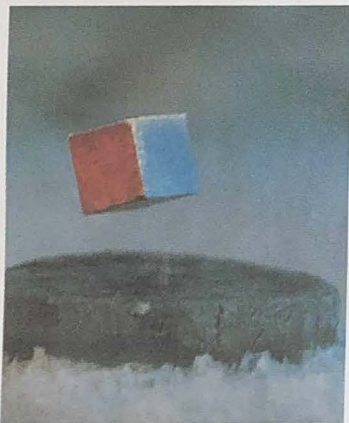
Photograph of a small permanent magnet levitated above a disk of the superconductor \text{YBa}_2\text{Cu}_3\text{O}_7 , which is at 77 K. This superconductor has zero electric resistance at temperatures below 92 K and expels any applied magnetic field. (Courtesy of IBM Research Laboratory)
