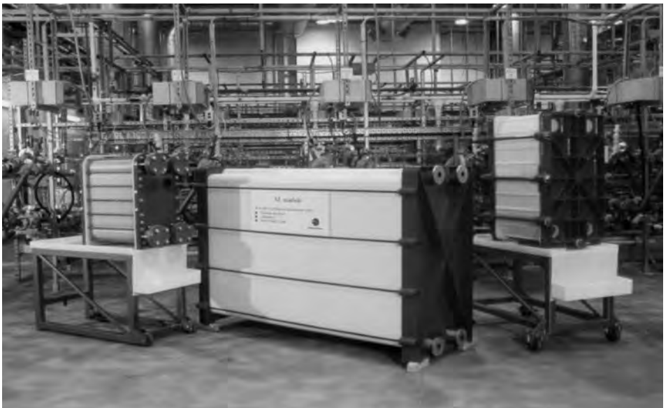
FIGURE 37.7 Regenesys modules of varying sizes. (From Ref. 25.)
