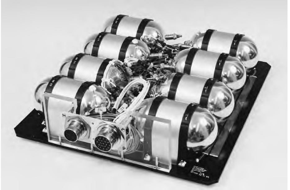
FIGURE 32.24 Mars Global Surveyor 23-Ah CPV battery assembly.
