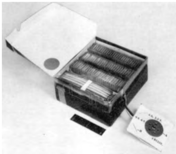
FIGURE 17.22 Magnesium/cuprous chloride radiosonde battery. Size: 10.2 \times 11.7 \times 1.9 cm; weight: 450 g, rated capacity: A_1 section—1.5 V, 0.3 Ah; A_2 section—6.0 V, 0.4 Ah; B section—115 V, 0.08 Ah.
