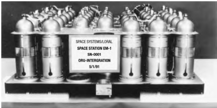
FIGURE 32.8 International Space Station 81-Ah Ni-H 2 38-cell assembly.
