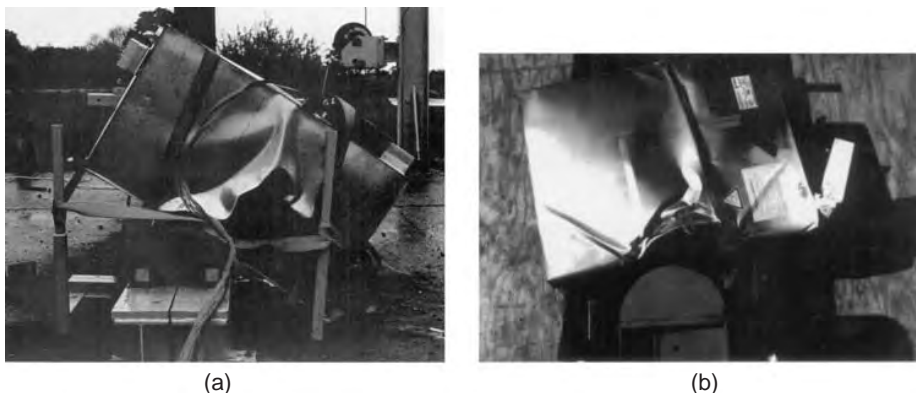
FIGURE 40.18 Two sodium-beta batteries following safety/abuse testing that was performed while the batteries were charged and at operating temperature: (a) an SPL HP sodium/sulfur battery dropped onto a steel pole, and (b) a Zebra battery after a steel beam was pushed through its mid-section ( Photograph (b) is courtesy of MES-DEA SA ).
