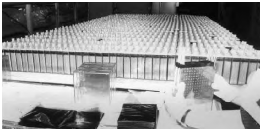
FIGURE 33.2 Cell stack being assembled into cell case; model LR-190, 210-Ah silver-zinc battery. (Courtesy of Yardney Technical Products, Inc.)
