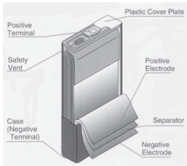
FIGURE 35.31 Schematic drawing of a wound prismatic cell. (Courtesy of Japan Storage Battery Co., Ltd.)
