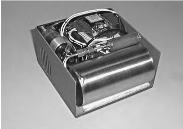
FIGURE 43.8 Metal hydride fueled system using BA-5590 type case. (The figure is of a system design having larger dimensions than the BA-5590.)
