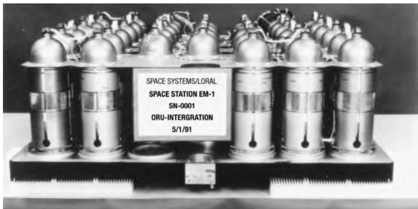
FIGURE 32.8 International Space Station 81-Ah Ni-H 2 38-cell assembly.
