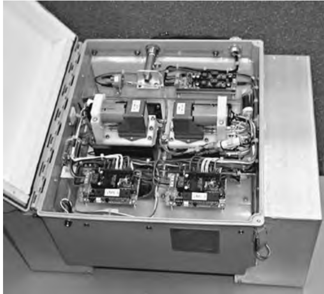
FIGURE 43.12 Twin 50-watt fuel cell systems. (Courtesy H-Power Corp.) Dimensions (cm): 33.0(H), 40.6(W), 45.7(L). Weight: 13.6 kg.
