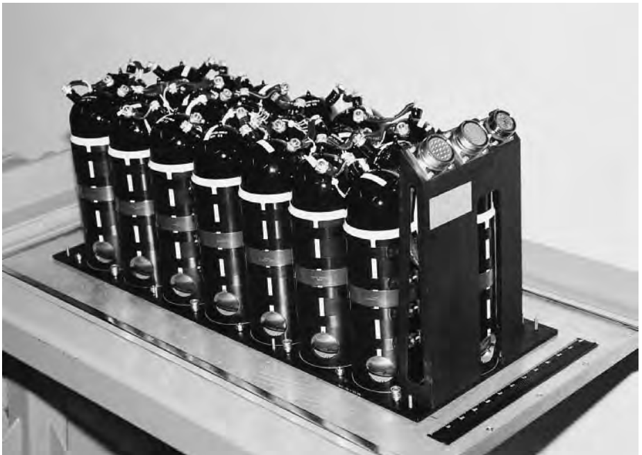
FIGURE 32.6 DMPS 100-Ah Ni-H 2 battery assembly.
