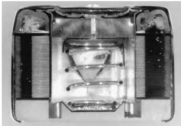
FIGURE 19.1 Cross-section of lead/fluoboric acid/lead dioxide multi-cell reserve battery showing “dashpot” cutter for copper ampoule. (Courtesy of U.S. Department of the Army.)
