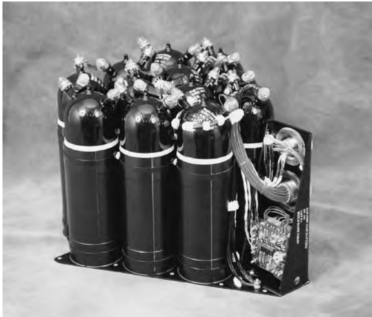
FIGURE 32.25 Mars Polar Lander 16-Ah CPV battery assembly.
