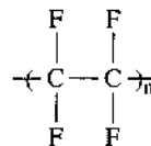
Figure 7.8 Polymer repeating unit for polytetrafluoroethylene (PTFE).
