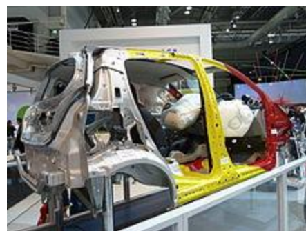
Body in white, partially outfitted to highlight the safety systems fitted to the vehicle.
