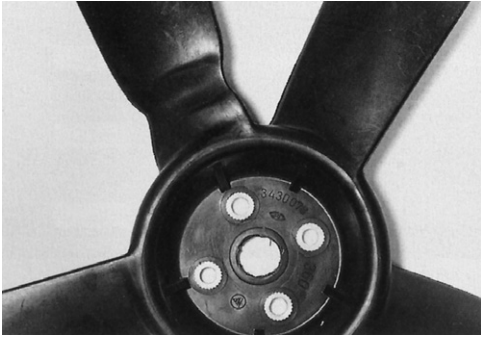
Figure 10.20 Necking of a polyethylene automotive fan blade [11]
