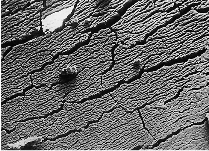
Figure 10.70 Surface of a polyoxymethylene specimen irradiated with ultra-violet light for 100 h in a laboratory environment
