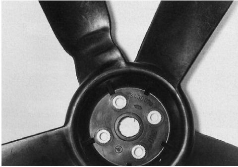
Figure 10.20 Necking of a polyethylene automotive fan blade [11]
