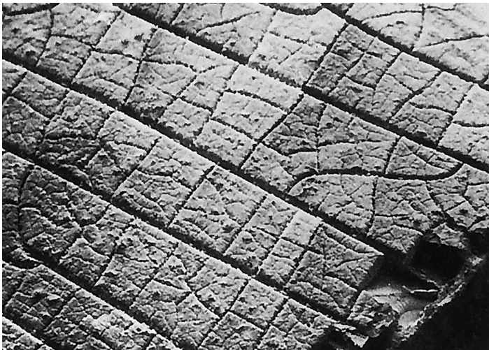
Figure 10.69 Electron micrograph of the surface of a high density polyethylene beer crate after nine years of use and exposure to weather
