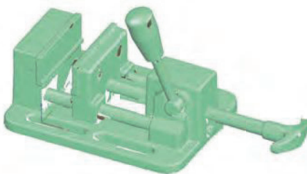
Scan data of the vise seen directly in Geomagic Spark’s capture window.
