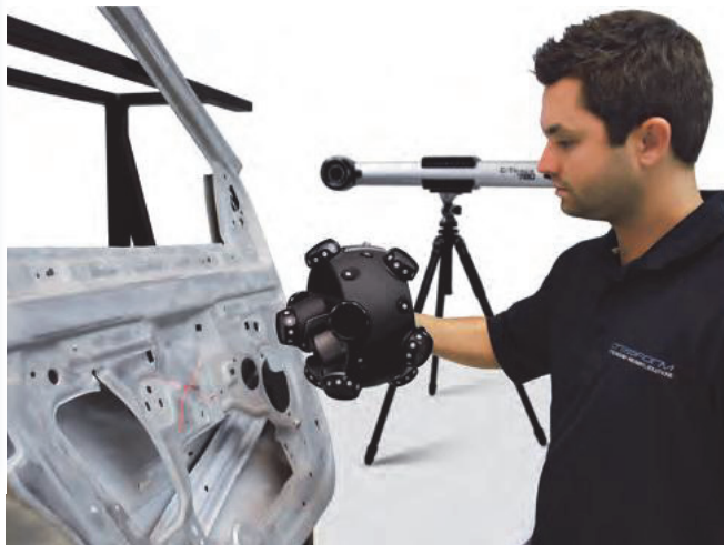
Optical CMM scanners like Creaform’s arm-free, handheld MetraSCAN tackle metrology or large-scale reverse engineering applications by promising to extend measurement volumes without loss of accuracy. Image courtesy of Creaform.
