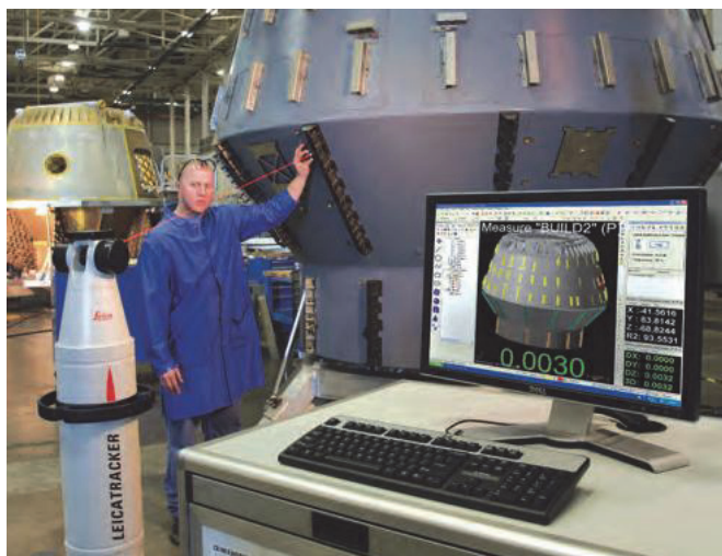
Computer monitor shows Verisurf Software controlling the Laser Tracker portable CMM used to inspect the SpaceX Dragon capsule. The software displays the in-tolerance deviation between the capsule and its respective CAD model in real-time to determine whether the capsule is assembled within specifications. Image courtesy of SpaceX.
