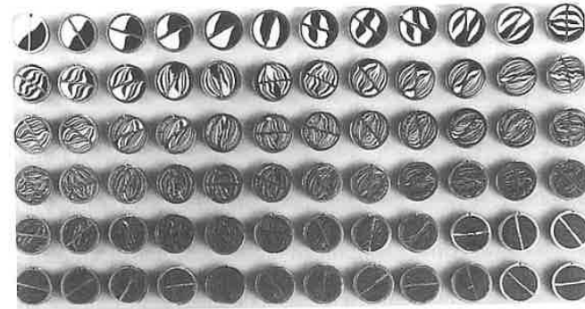
Figure 6.37 Experimental progression of the layering of colored resins in a Kenics static mixer.
