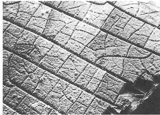
Figure 10.69 Electron micrograph of the surface of a high density polyethylene beer crate after nine years of use and exposure to weathering.
