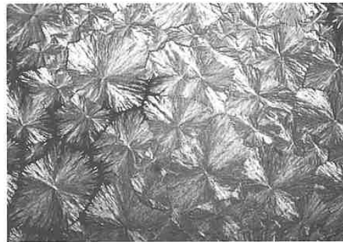
Figure 13.10 Electron micrograph of permeating media through the interspherulitic boundaries of polypropylene.
