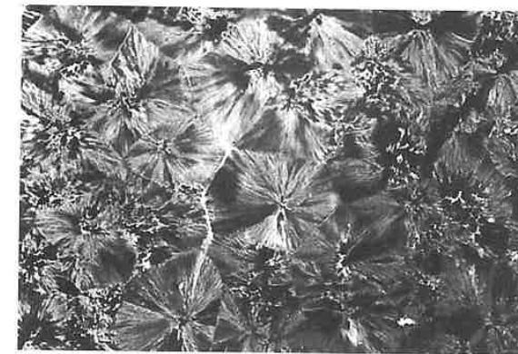
Figure 10.16 Micrograph of crack formation at inter-spherulitic boundaries (polypropylene).
