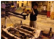
1 3D scanning of stamping die in production
