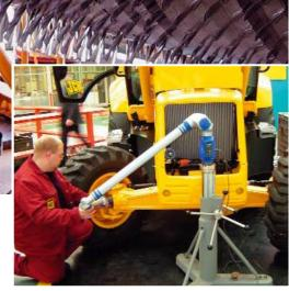
arge construction machines are too big for conventional measuring devices. With the help of a FaroArm, which allows measurements to be made directly in situ. Costly transport of large, heavy components or assemblies to measuring devices is eliminated.
