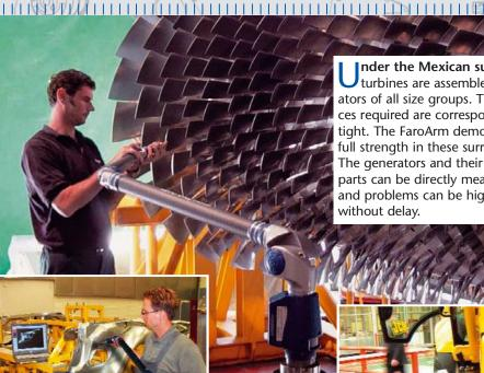
Inder the Mexican sunshine ABB turbines are assembled for generators of all size groups. The tolerances required are correspondingly tight. The FaroArm demonstrates its full strength in these surroundings. The generators and their component parts can be directly measured in situ and problems can be highlighted without delay.
