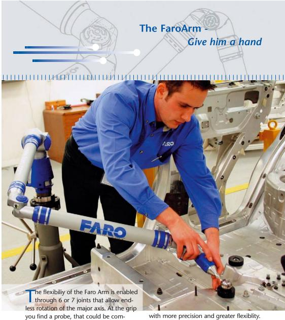
through 6 or 7 joints that allow endless rotation of the major axis. At the grip you find a probe, that could be compared to a forefinger. To measure a point the probe is placed on the measurement position.
