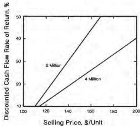
Figure 10.20 Price sensitivity analysis for thermoform molding of crystallized polyethylene terephthalate, CPET trays at year 5
