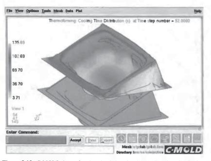
Figure 3.12. C-MOLD thermoforming simulation showing cooling time distributions for a sheet formed over a tub mold. The black-and-white reproduction limits the original's perceptibility (courtesy of AC Technology North America, Inc., Louisville, KY 40223).
