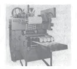
Figure 7.17. High speed automatic thermoformer and stacker (courtesy of Adolf Illig Maschinenbau GmbH & Co., D-74080 Heilbronn, Germany).
