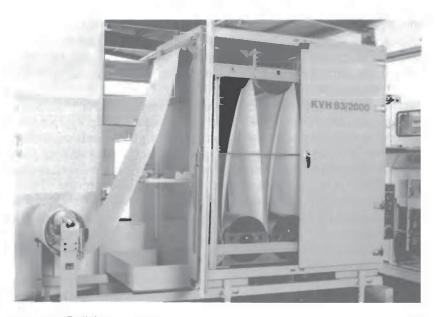
Figure 2.9. Roll-fed material preheating station (courtesy of Paul Kiefel GmbH, D-83395 Freilassing, Germany).
