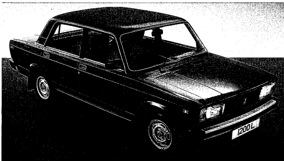
← This is a British market 1986 Lada Riva 1200L, based on the 1,198cc VAZ 21051. (Author's collection)
