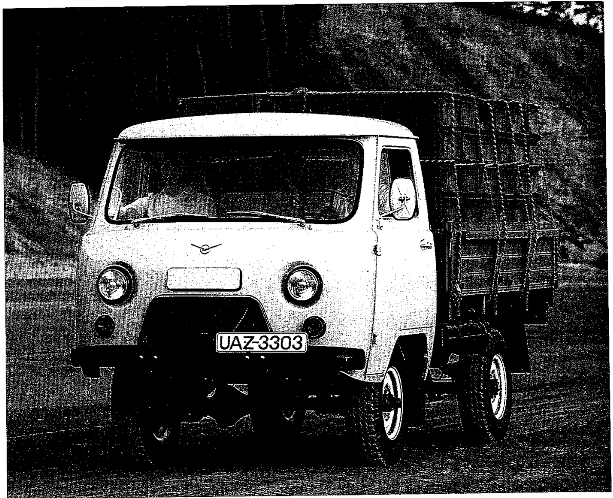
↑ The drop-side pickup continued as the UAZ 3303, complete with its wooden body. (Author's collection)
