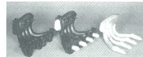
Figure 9.9 (Left) An intake manifold made from glass-fiber-reinforced polyamide 66 by fusible core technique; (center) core overmolded with plastic; (right) fusible core cast from bismuth-tin alloy [30]. Source: BASF. (From Innovation in Polymer Processing—Molding , Stevenson, J. F., (Ed.) (1996), Hanser, Munich, p. 155, Fig. 4.3.)
