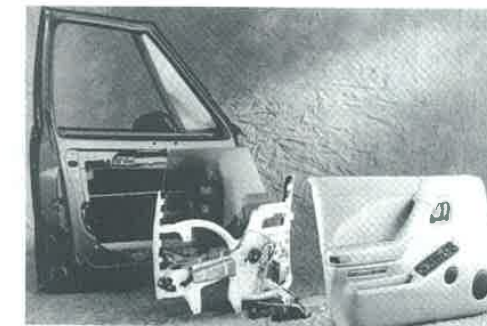
Figure 9.16 Automotive door modules (Courtesy of Delphi Interior & Lighting Systems) [25]. (From Injection Molding Alternatives—A Guide for Designers and Product Engineers , Avery, J. A., (1998), Hanser, Munich, p. 97, Fig. 5.3.18 and p. 98, Fig. 5.3.19.)
