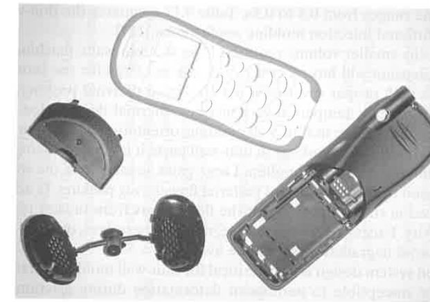
Figure 9.64 Plastic housings and components of cellular phones (Parts courtesy of Flambeau Micro, Sun Prairie, Wisconsin, USA). The cellular phone on the top was overmolded with thermoplastic elastomer to provide soft touch feeling and drop protection. (Part courtesy of Yomura Company Ltd., Taiwan.)
