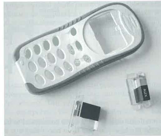
Figure 9.42 (Top) TPE (thermoplastic elastomer) overmolded on ABS/PC for a mobile phone to provide soft touch feeling and drop protection. (Bottom) Black color ABS with transparent acrylic, used on audio push button for light on transmitting. (Parts courtesy of Yomura Company Ltd., Taiwan.)
