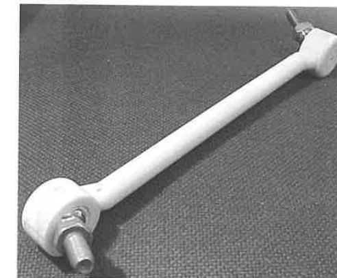
Figure 9.48 A car stabilizer component using a hybrid push-pull and gas-assisted injection process. The material is a partial aromatic polyamide (polyarylamide) with 50% short glass fiber content. (Photo courtesy of StructoForm GmbH, Aachen, Germany.)
