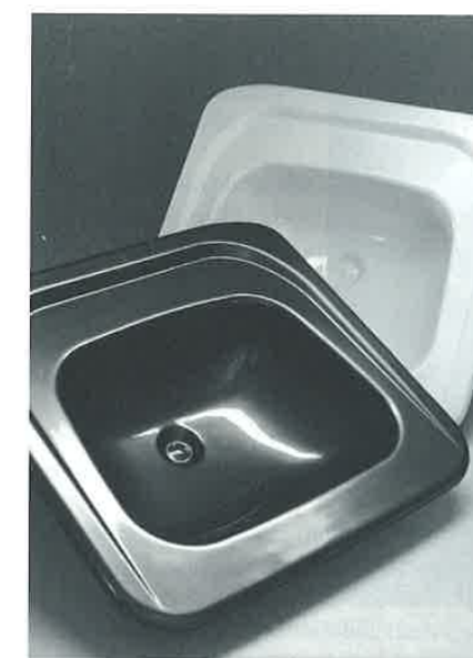
Figure 9.36 Lavatory sink molded with Inverted Force Molding (IFM), which permits high gloss decorative films to be molded across the entire surface without damage or distortion of color on deep draws of film. (Courtesy of Hettinga Technologies, Inc., Des Moines, Iowa, USA.)
