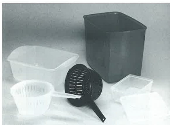
Figure 9.34 An assortment of thin-walled kitchen-ware molded from high-density linear polyethylene, HDLPE. Each part was produced using the Inverted Force Molding (IFM) process on a 275-ton press. (Courtesy of Hettinga Technologies, Inc., Des Moines, Iowa, USA.)
