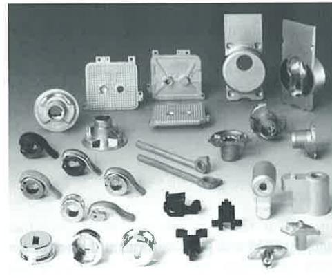
Figure 9.52 A range of powder injection molding components [104].
