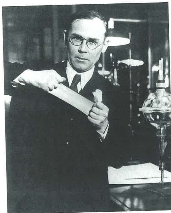
Figure 2.9 Wallace Carothers stretching a sheet of polychloroprene.
