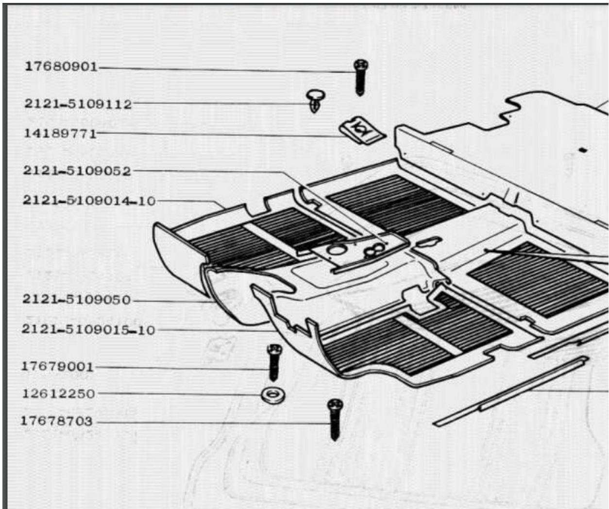
14. Another portion of the footwell of the Lada Niva is made up by the floor tunnel cover. This is part of main floor structure of the Niva and also did not change between 1977 and 1993. It is shown on page 104 of Exhibit B and the part number is 2121-5109050. The picture in the prior paragraph shows this part as well.
