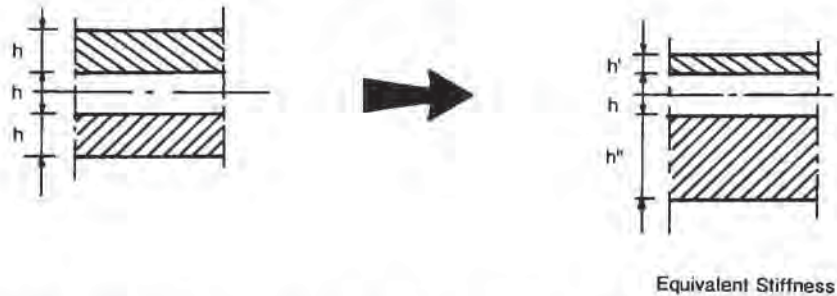
Figure 9.27 Equivalent stiffness concept for three-ply laminate. (Left) Actual thicknesses of laminate. (Right) Effective thicknesses when plies vary in modulus
