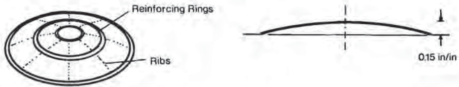
Figure 7.86 Using doming, reinforcing rings and/or radial ribs to minimize optical distortion, eversion in thermoformed disks
