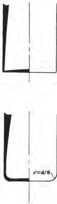
Figure 7.8 Draw-down into (top) sharp-cornered cylinder and (bottom) radiused cylinder. Corner radius, r' = d/8 , where d is cylinder diameter
