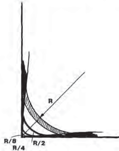
Figure 7.13 Progressive draw-down into two-dimensional corner
