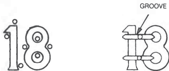
Figure 3.17. Mold details for raised characters. Small circles show air vent holes.
