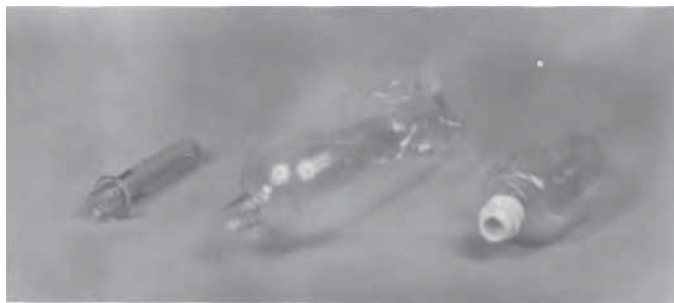
Figure 8.2. Stretch-blow molded polyester bottle: (left) injection molded preform, (middle) blown bottle, and (right) much of the elastic stretch recovered and neck part crystallized on reheating.
