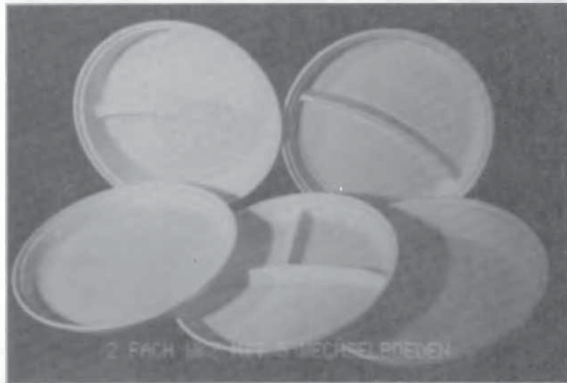
Figure 3.9. Plates formed in molds with quickly interchangeable bottoms (courtesy of Gabler Maschinenbau GmbH, Luebeck D-23512, Germany).
