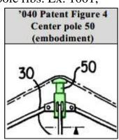
Rake admitting the "center pole extends above the center pole ribs"). As shown in Fig. 4, by extending vertically above the ribs, the center pole stretches and sustains the tent's roof.<sup>1</sup> By contrast, a center pole that extends downward to the ground (such as that contemplated in the discussion of the prior art in Yang (Ex. 1004, 4)) would serve as a support column for the frame but would not stretch and sustain
