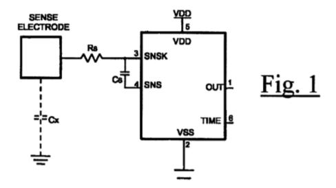
Figure 1 "schematically shows sense electrode connections for an example chip for implementing an auto-off function." Ex. 1001, 3:13–15.
