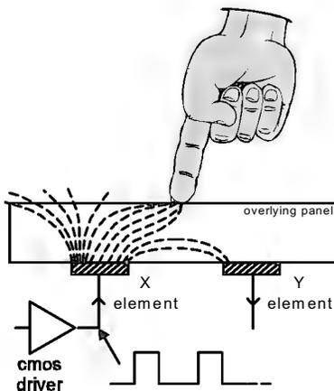
Burst mode operation permits the use of a passive matrix, reduces RF emissions, and provides excellent response times.
