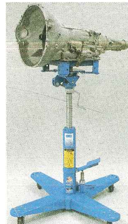
Fig. 4-13. Transmission jack is designed for removing, transporting, and installing transmissions when using an overhead lift. Hydraulic lift is foot operated and raises to height of 72 in. (OTC Div. of SPX Corp.)
