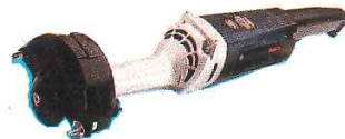
Fig. 4-7. Die grinder with a high speed stone installed. This tool is used for removing burrs and for other smoothing operations. (Robert Bosch)
