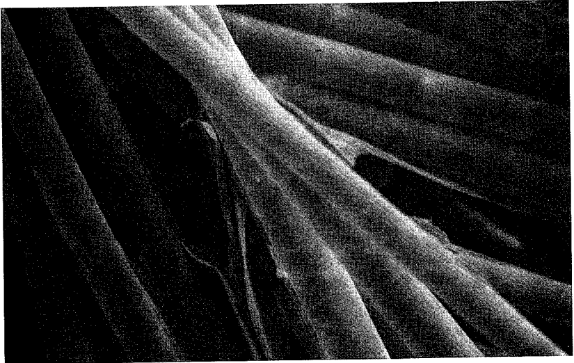
FIGURE 2.5.2-3 Photomicrograph at higher magnification of the fibers used to construct the glass-mat insulator used in the NEW CIGARETTE. The sheets of pectin binder can be seen between the strands of glass.
