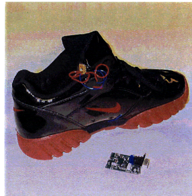
PAN transmitter and PAN III RS232-to-body modem.
