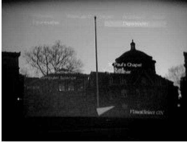
Figure 2. View shot through the see-through headworn display, showing campus buildings with overlaid names. Labels increase in brightness as they near the center of the display.
