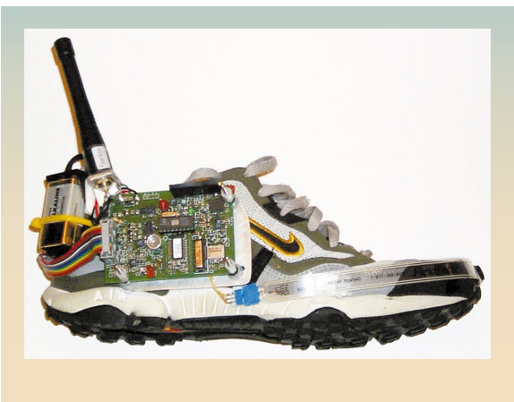
Figure 4 The modern, perfected shoe with protective electronics cover removed
