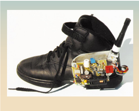
Figure 4 The modern, perfected shoe with protective electronics cover removed
