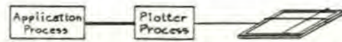
Fig. 2. Two processes using the plotter protocol. The application sends messages to the plotter process that completely describe the figures to be plotted. The two processes may execute on separate computers linked by a network, or on a single computer that provides message communication between the two processes.
