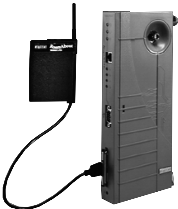
RoamAbout 2.4 GHz Frequency Hopping (FH) PC Card in Digital's RoamAbout Access Point
