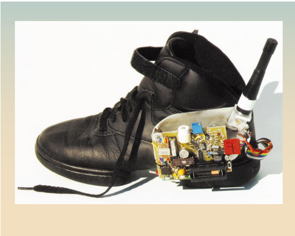
Figure 4 The modern, perfected shoe with protective electronics cover removed
