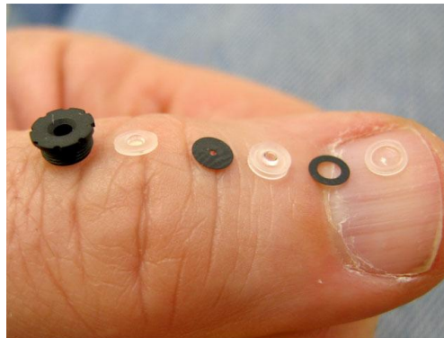
Fig.2: 3-element lens, disassembled. Barrel, three plastic aspheric lenses, thin sheet aperture stop and baffle.
