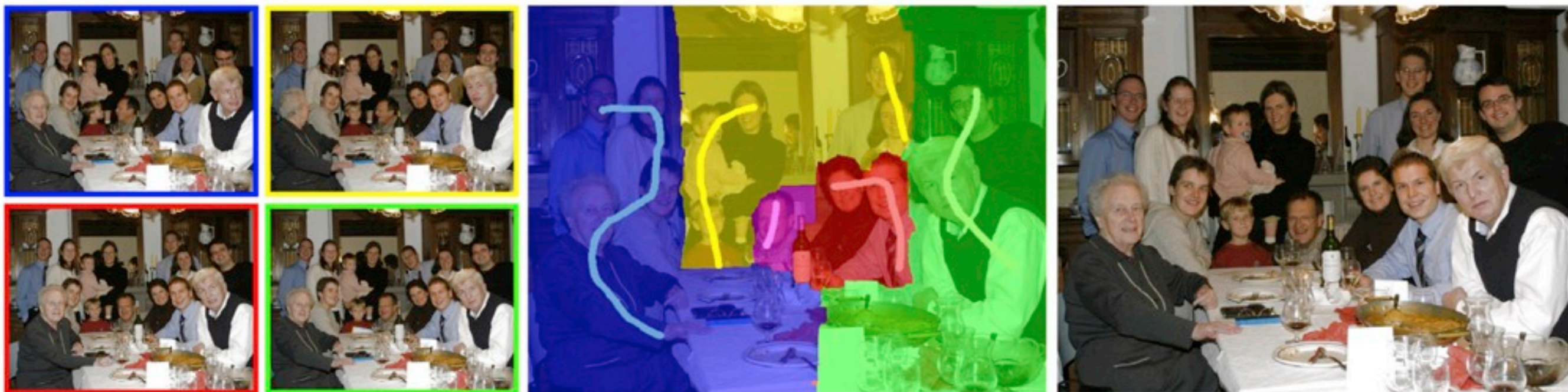
Figure 1 From a set of five source images (of which four are shown on the left), we quickly create a composite family portrait in which everyone is smiling and looking at the camera (right). We simply flip through the stack and coarsely draw strokes using the designated source image objective over the people we wish to add to the composite. The user-applied strokes and computed regions are color-coded by the borders of the source images on the left.
