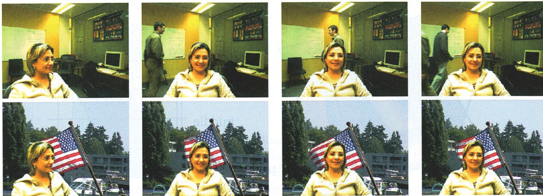
Figure 11.14 Background replacement using z-keying with a bi-layer segmentation algorithm (Kolmogorov, Criminisi, Blake et al. 2006) © 2006 IEEE.
