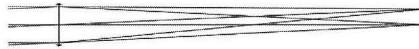
Figure 2.11 First-order layout of the doublet lens. Two light beams are shown for the on-axis field point and for the 5 degrees off-axis field point.
