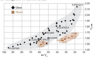
Plastic provides a distinct cost and weight advantage and an excellent ability for forming complicated surfaces and integrated features. Disadvantages of plastics include: high static buildup that attracts foreign particles and can lower cosmetic surface qualities, high thermal expansion, and high temperature coefficient of refractive index. Plastics cannot be cemented or coated as easily as glass.
