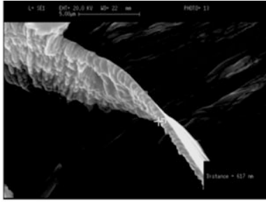
(a) (001) cutting plane; Depth of cut = 5 \mu\text{m}
