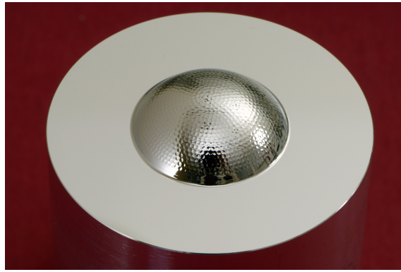
Figure 8. Free-form lens array mold insert containing 1,219 single spherical lenslets whose vertices are arranged on a hemisphere
