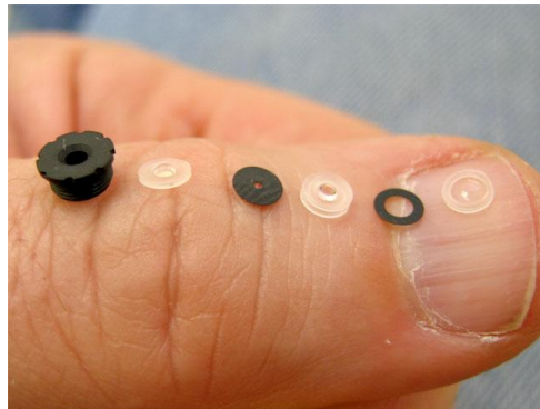
Fig.2: 3-element lens, disassembled. Barrel, three plastic aspheric lenses, thin sheet aperture stop and baffle.
