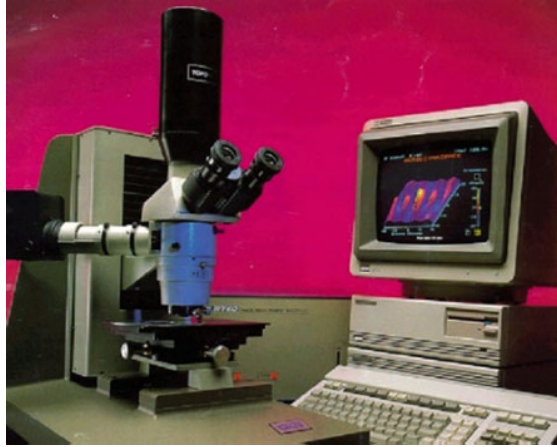
Fig. 4.6 Wyko noncontact microsurface measurement system
