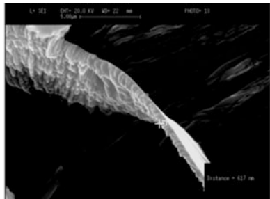
(a) (001) cutting plane; Depth of cut = 5 \mu\text{m}
