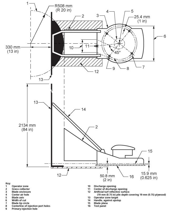
Figure 12g - Views of rear discharge pedestrian-controlled mower with grass collection system
