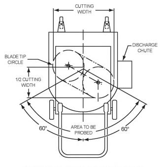
FIGURE 4 - AREA TO BE PROBED MULTI-BLADE MOWERS (2) For a mower with a swing-over handle, the areas to be probed shall be determined as in paragraph (b) (1) (ii) (A) (1) of this section from both possible rear positions. (See Fig. 5.)
