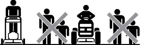
Ref ANSI B71.1 2003 (derived from ISO 11684 Figure B.2.6 and section D.9 - communicating idea of prohibited action or hazardous location)
