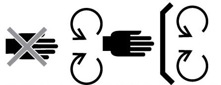
Ref ISO 11684 B.2.11 for "Do not open or remove safety shields while engine is running." Avoidance graphic is derived from B.2.11.
